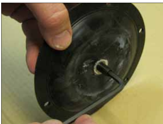
Fig 6.13. Mount the pin screw (part of the diaphragm shaft pos 16) securely in the diaphragm (15) by means of an allen key.
