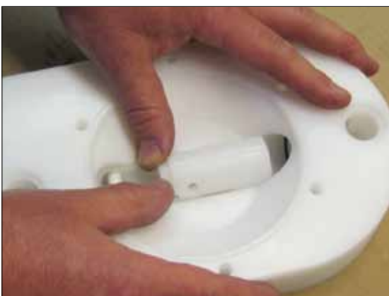
Fig 6.19. Place the spacer sleeve (19) upside down and press it up towards the the upper valve seat (20).
