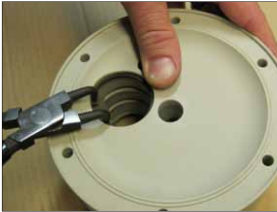
Fig 6.1. Mount the circlip (27) on one side.
