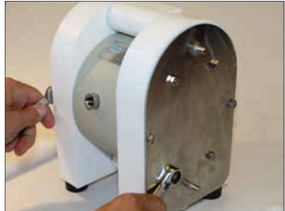
Fig 5.2. Unscrew the housing nuts (37). Carefully pull out the pin screws (14). Lay the pump with one housing facing down and carefully lift the loose housing (11). Proceed as in fig 5.3.
