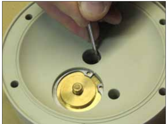
Fig 5.12. If the shaft sealings (36) seem to be worn out (by internal leakage of air), carefully remove them with a pointed tool. During this operation, the sealing (36) and backup o-ring (47) usually get destroyed, so make sure to have replacement spares available.
