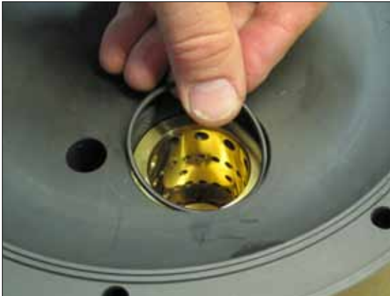
Fig 6.7. Place the last o-ring (pos 30) on the cylinder.
