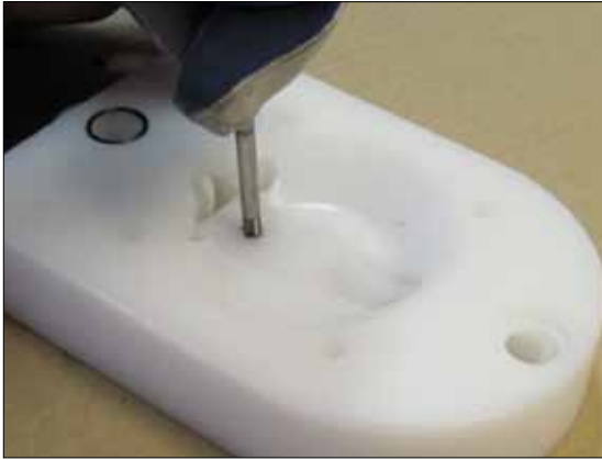
Fig 5.9. Screw a pinscrew into the hole of the spacer sleeve (19). On newer models of TR9 this hole does not exist, then lift instead carefully by means of a screwdriver.
