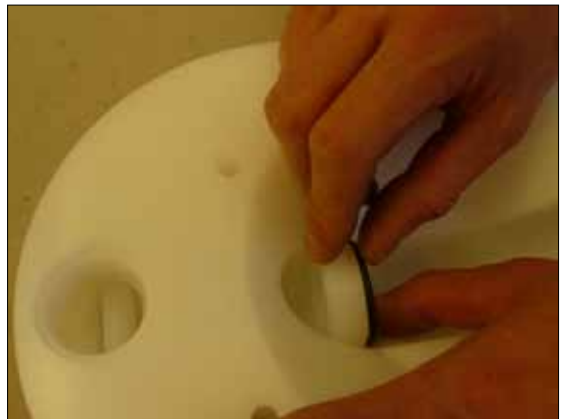
Fig 6.18. Mount the valve seat O-ring on the bottom of the valve seat (222) and push seat assembly into the housing (11)
