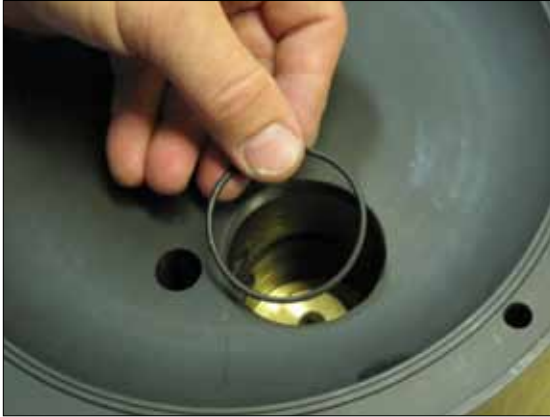
Fig 6.5. Place one of the o-rings (pos 30) on the endcap.
