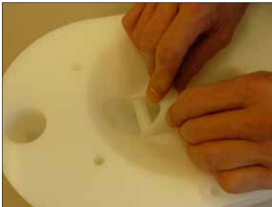
Fig 6.17. Mmount blocking pin (2021) in special cut in pump housing. Fix the ball stop (22) in upper sleeve and mount it in the pump housing.
