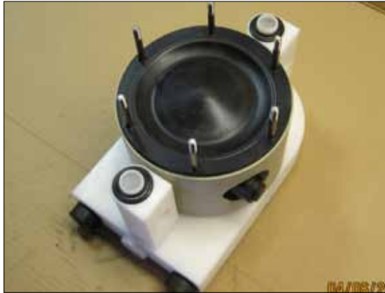
Fig 6.25. Put on the inlet and outlet connections (13), make sure all o-rings (18) are mounted.
