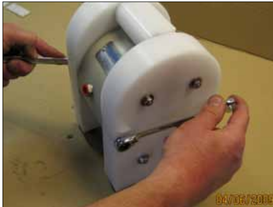
Fig 6.27. Fasten the nuts (37) alternatingly, with or without washers depending on how much of the thread comes out. If some of the nuts were fastened without washer, unscrew those and put washers underneath. Tighten the nuts according to recommended tightening torques in chapter 5.
