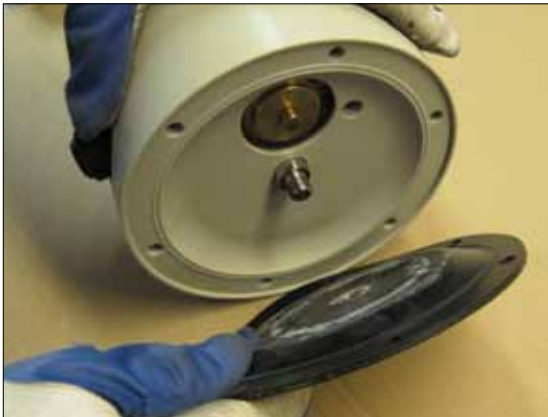
Fig 5.11. Press the diaphragms (15) to their neutral position (both have the same distance to the center block). Hold one of the diaphragms (15) and unscrew the other. Then pull out the remaining diaphragm (15) with the diaphragm shaft (16).
