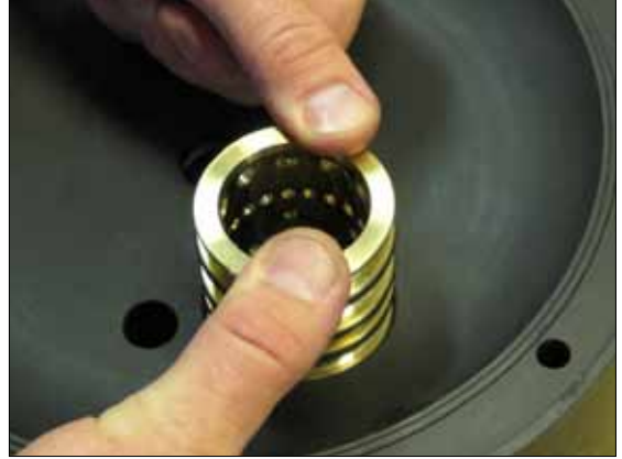
Fig 6.6. Make sure all four o-rings (pos 30) are mounted on the cylinder. Use a little water on the o-rings to easier slide the cylinder into the centerblock. Other lubricants should not be used.
