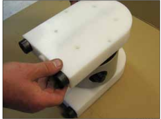
Fig 6.26. Carefully lift on the remaining housing.
