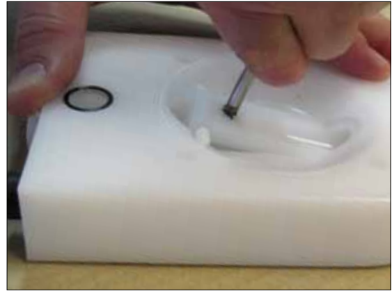
Fig 5.10. Lift and pull down the spacer sleeve (19).
