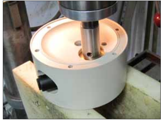
Fig 5.14. Press out the air valve (61) by means of a pressing device. Be careful not to damage the brass edges of the air valve.
