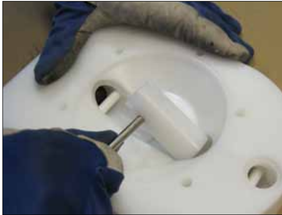
Fig 5.6. Carefully pull out the the spacer sleeve (19). Please note that force never shall be used by for dismantling.
