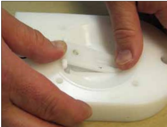
Fig 6.22. First insert the lower rod valve (21) and upper rod valve (20). Push the spacer sleeve (19) with its pin (22) into the housing (11). You may need to knock gently with a plastic hammer.
