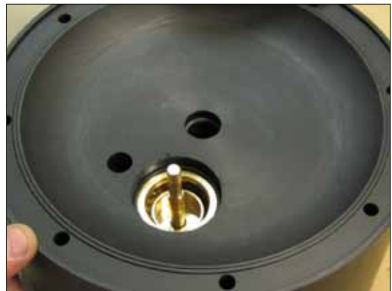
Fig 5.16. Now when both endcaps are removed, push out by hand the shaft and piston.
