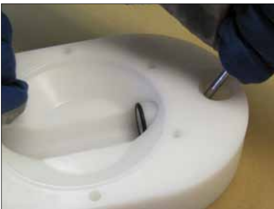
Fig 5.8. Push out the upper sleeve (202), to remove valve seat assembly and remove blocking pin (2021)
