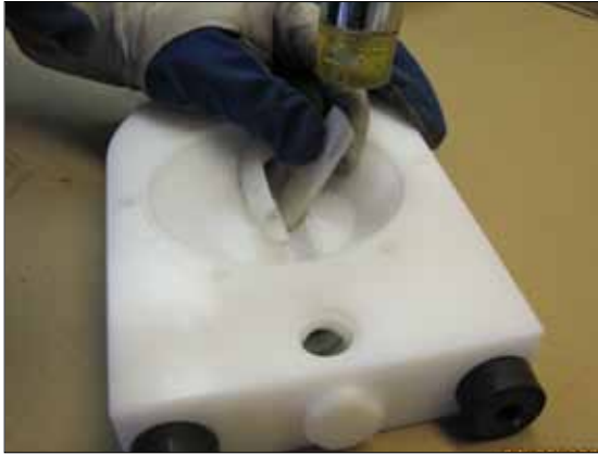
Fig 5.4. To remove the spacer sleeve (19), use a piece of plastic and a hammer to carefully knock to turn it.
