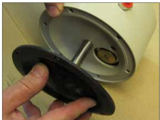
Fig 6.14. Mount the diaphragm shaft (16) on the diaphragm (15) and push the assembly carefully through the hole in the centerblock (12).
