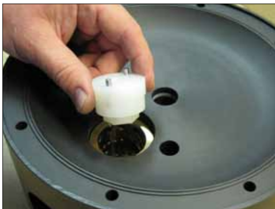
Fig 5.17. To push out the cylinder, use the other side of the mounting tool that fit into the cylinder.
