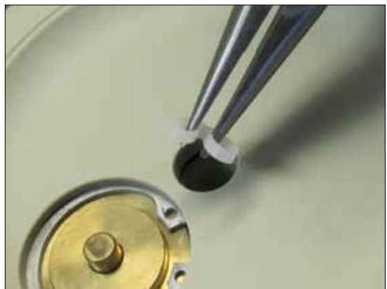
Fig 6.12. To mount the shaft seal (36), bend it to a kidney shape and insert carefully to the groove.
