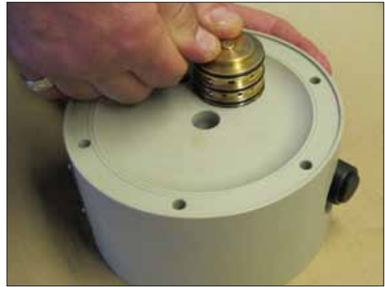
Fig 6.2. Put a little water on the o-rings (30), other lubricants should not be used. Carefully push the air valve (61) into the housing. Mount the circlip (27) on the remaining side (see fig. 6.1).
