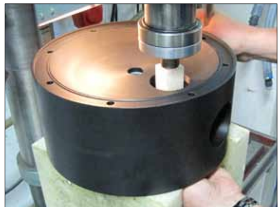
Fig 5.18. Press out the cylinder, be careful not to damage the edges of the cylinder.
