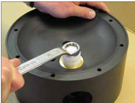
Fig 5.15. Carefully unscrew the air valve endcap by means of the mounting tool (282). Do the same with the endcap on the other side.
