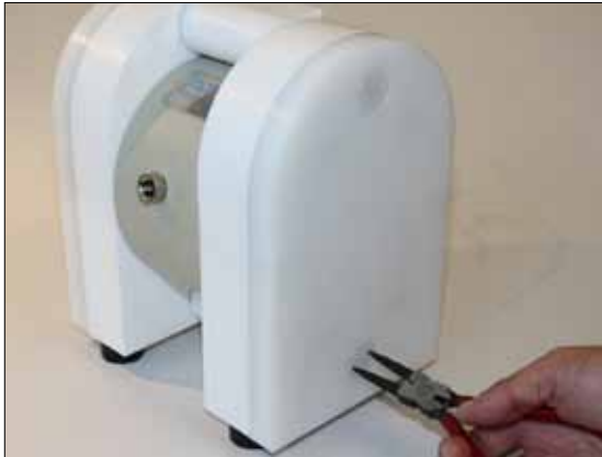
Fig 5.1. Unscrew the plugs (571) by means of a circlip plier. Carefully lift off the PE covers (1181).
