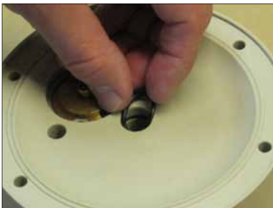
Fig 6.11. Insert the shaft seal o-rings (47) in the groove.
