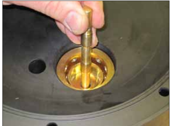
Fig 6.8. Carefully mount the piston and shaft by hand. Repeat steps Fig 6.3 and Fig 6.4 on the remaining side. Carefully secure the endcaps equally on both sides.
